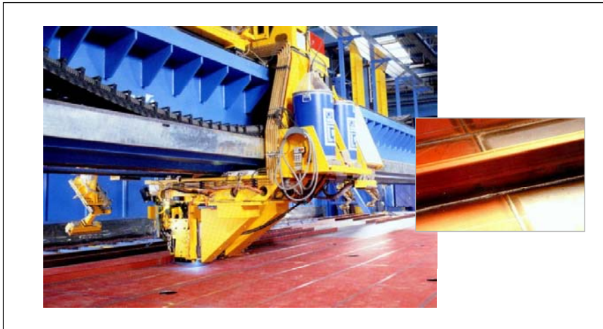
Fig. 8 CO 2 -Laser-GMA-hybrid welding from panels and stiffeners at shipyard “Meyer-Werft” in Papenburg, Germany [4]
